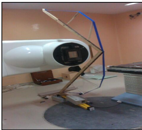
FIG 4: MEASUREMENT POINTS FOR ON POSITION LEAKAGE IN OTHER THAN PATIENT PLANE
