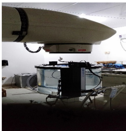
Figure 4 Radiation Field Analyser measurements in Theratron 780E to get beam profiles.
