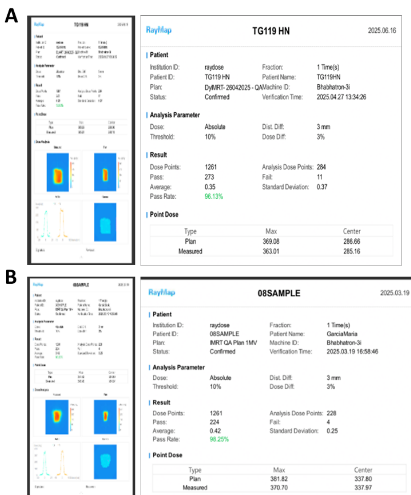
Figure 7. Illustration of fluence patterns with two-dimensional map check phantom measurements for (A) head and neck plan and (B) prostate plans
