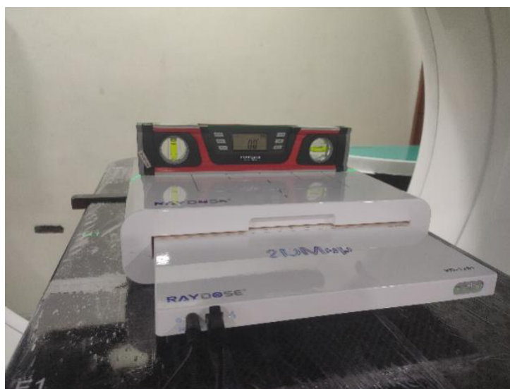
Figure 3. Array detector (two-dimensional map matrix/RayMap) kept in the O-ring gantry for quality assurance measurements
